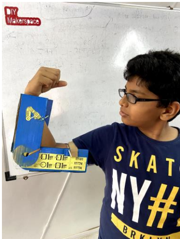
Figure 5 and 6: Version 1 of the EXO- Arm designed by the students at the end of the pilot . The sensor assembly which is on the outside of the students arm to detect muscle movements of the students.
